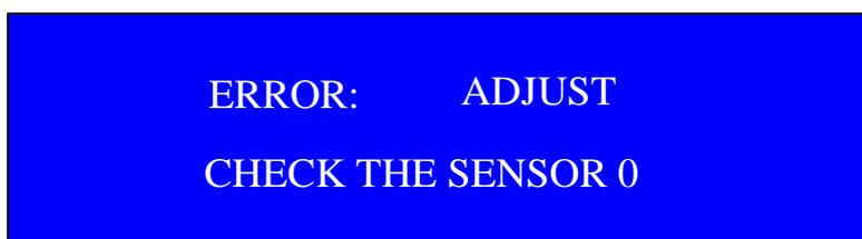
·When it displays ERROR ADJUST, it means the signal of alloy sensor is abnormal, the self-test can not be done normally, please contact your local distributor for solution.
