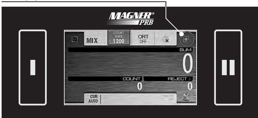
1.2 Keys «I» or «II» are used for the start of count in the manual start mode. To start, press the button of the active user.
