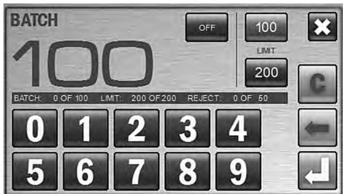
You can enter **BATCH** mode by pressing the key (for the batch size > 0) and disabled by pressing the key. By pressing the key you cancel the unsaved changes and exit to the main menu. The batch size is set with the numerical keys. Any batch size since 1 until 999 is available. Key is used to clear the current batch size. Single pressing of the key deletes the digit from the right to the left.
