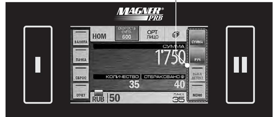
In the extended visual mode, the highlighted parts are not only the active user's key but also the check-box in the upper corner of the screen. The figures given below show the control panel appearance for various users: at Figure 33 is for 1st user (I), at Figure 34 is for 2nd user (II).
