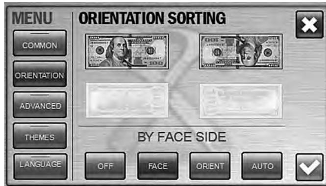
**ORIENT:** the banknotes placed into the hopper with their faces up and readable from the left to the right serial number (upside up) will get into the stacker (see Figure 23). The other banknotes will be transferred into the reject pocket.
