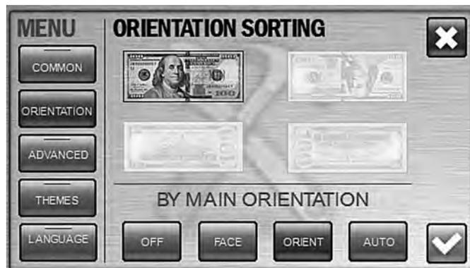
**AUTO:** The banknotes with the same orientation as the first counted banknote in a batch (see Figure 24) will get into the stacker. The other banknotes will be transferred into the reject pocket.
