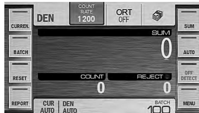
In the **BATCH** submenu a user can change the stacker capacity. The current value of the stacker capacity is highlighted in blue (see Figure 47).
