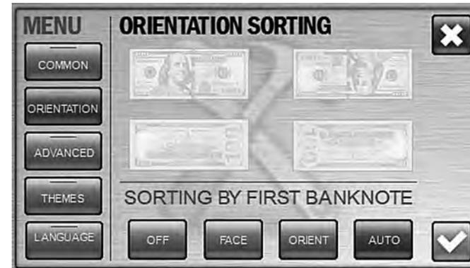
To get an access to the orientation sorting, press the hot keys « **ORT** **OFF** » (see Figure 25). By pressing **ORT** key, the dropdown menu «orientation sorting» appears. The required orientation may be selected by a repetitive pressing of the key **ORT** **OFF**; in this case, the modes will be selected in turn:
