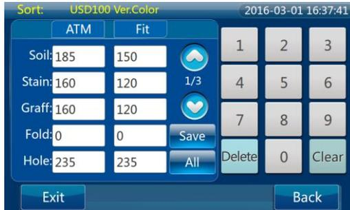
Notes: The sorting parameters totally include following the 13 items: Soil, Stain, Graffiti, Tape, Fold, Hole, Missing Corner (M-C), Dog-ear, Missing Edge (M-E), Tear, Wrinkle, Watermark, Deinked, the parameter setting range is 0-255 and the corresponding parameters of the same Fit Banknotes should not be greater than the parameters ATM Banknote.
