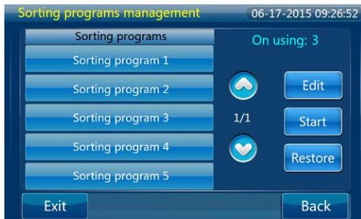
There are five sorting programs in total, and the default sorting program is among 1~5. The sorting parameter grades that correspond with each sorting program are from high to low, that is, the sorting program 1 is the strictest and the sorting program 5 is the loosest.
