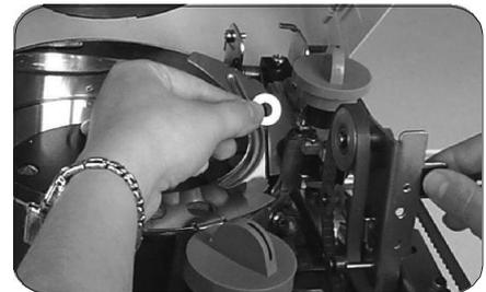
Restore the thickness adjustment Block and Front Feed Pulley Arm, close the Top Cover.
