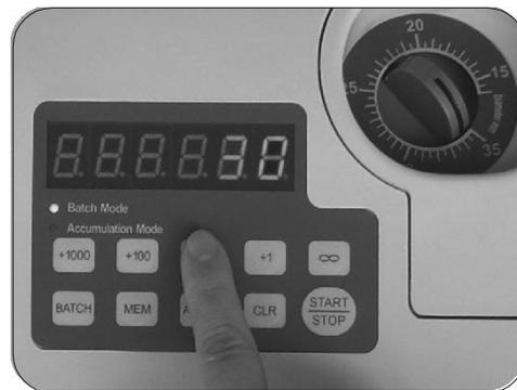
Press **MEM** key, save the amended default batch quantities in the memory, the previous default batch quantities will be replaced;
