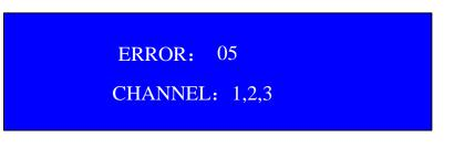
•When it displays such error message, it means there is short circuit point on the coin outlet drawer full warning sensor. Please check the coin outlet drawer and sensor connecting wires. After solving this problem, press CLR key to come back into main display modes interface.
