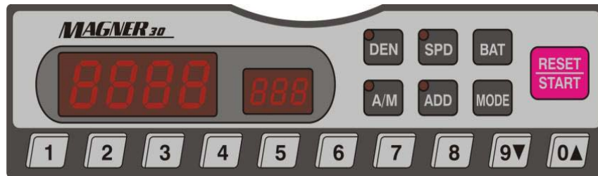
[ Control Panel for Simple Counter ]
