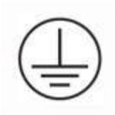
Grounding work should be made for safety and prevention of static electricity and noise failure. In addition, a ground wire should be installed independently without sharing the wire with other products. At grounding work, please be sure to contact our distributor near you or our designated dealers. In case of electrical leakage when grounding is insufficient or not connected, it may cause fire and/or electric shock.
