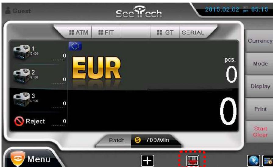
You can select Operation mode(Mix, SG and SP) with Serial reading by pressing below blue icon
