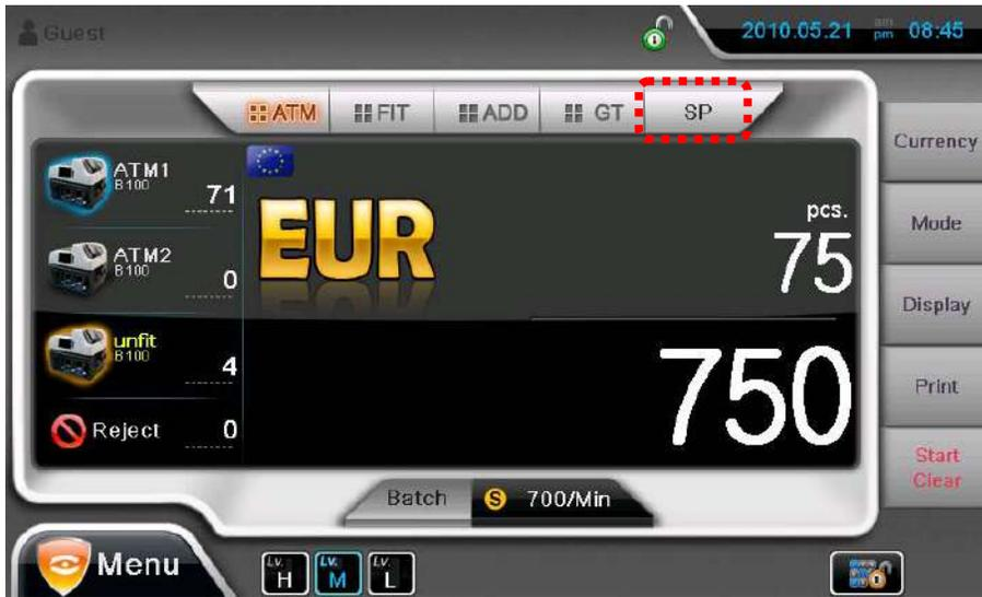
When ATM or FIT mode is off, the third recognized denomination is sent to Pocket 3.
